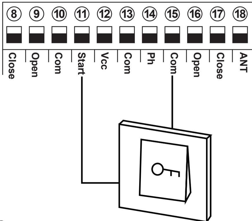
Terminal ⑪ and ⑮ are for connecting with the push button.
