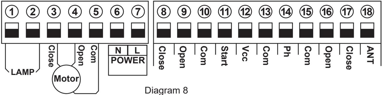
1&2. Lamp: used for connecting with flashing light, output voltage is AC 110V/ 220V.
