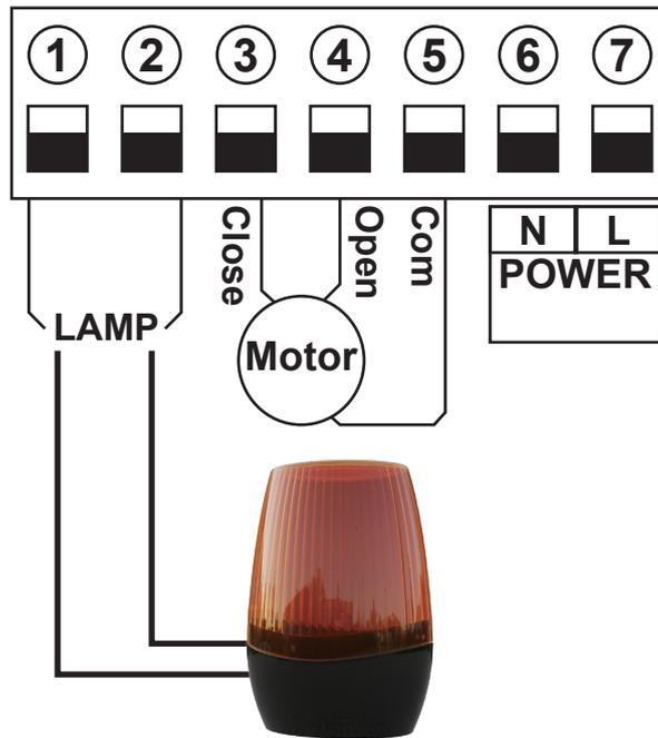
Terminal ① and ② are for connecting with the flash lamp .
