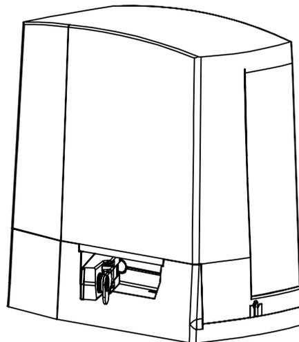
Releasing arm in torsion, wriggle 90 degree gate operator will be in releasing state
