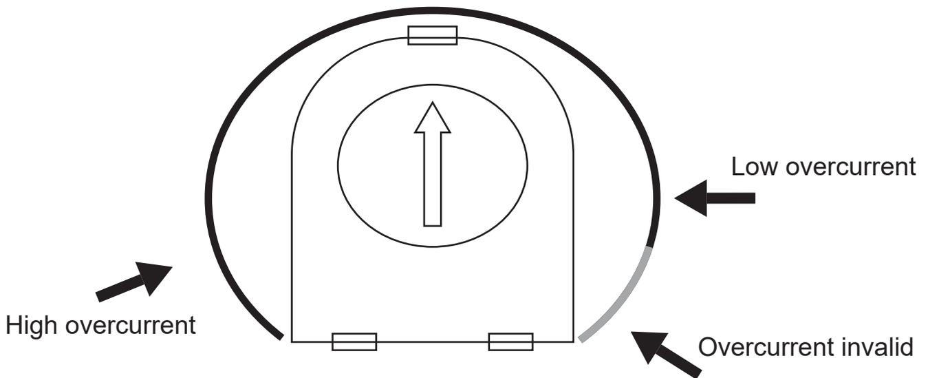
There are 2 potentiometer for " OPEN/CLOSE " overcurrent adjust to set the open and close overcurrent value separately.
